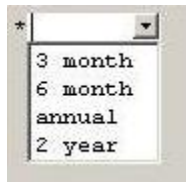
Figure 2-8: Example of a Drop-down List (list contents displayed but no choice made)
